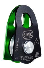
This mid-sized PMP is the perfect choice for rigging with 11 mm (7/16") rope or when you don't have room for a 3" PMP. Pulley will accommodate up to 13 mm rope.
