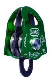
The SMC 2" Double Aluminum Prusik Minding Pulley "PMP" - NFPA is the perfect mid-sized choice for rigging with 11 mm (7/16") rope or when you don't have room for a 3" PMP. Pulley will accommodate up to 13 mm rope.
