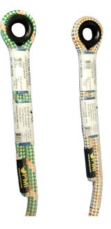
The Compact Sewn Termination for <u>11 mm PMI® Extreme Pro Rope</u> is available with either one or two ends. PMI uses precision stitching to create a permanent, sewn termination that is stronger than any knotted termination and nearly as strong as the rope itself. Heat shrink tubing protects the stitching and the label from abrasion.
