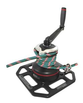
The Harken Traction Winch provides the user with a lightweight, CE certified, portable winch mounted to a robust adaptor plate. The Harken Traction Winch weighs 15.40 lbs (7.000 kg) with a 1/2 ton working load limit, the 2 speed winch magnifies the operator pulling power by up to 40 times. The multiple mounting options provide versatility when working in difficult or remote environments.
