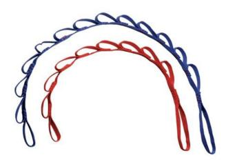
Constructed of 3/4 " (19.5 mm) Tubular Webbing, this multi-loop daisy chain helps organize your rigging gear. While not rated for life safety, each loop on our gear daisy will hold 2 kN (450 lbf) because of the "double back" construction.
