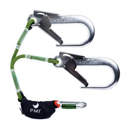
This V-shaped fall arrest lanyard incorporates an integral energy absorber, and complies with European fall arrest standards EN 355 and EN 362. If offers maximum protection for passing intermediate anchors on a fixed line. Sewn terminations are protected by a removable cover to permit complete inspection.
