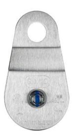
Based on Russ Anderson's original design, these pulleys are essential equipment for the serious rigger. Rotating side plates allow attachment of the pulley anywhere on the rope and the 3" and 4" models will accept multiple carabiners. Axle nuts are marked with a blue witness line to indicate if the axle nut has been turned or tampered with.
