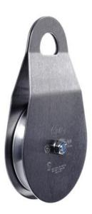
Based on Russ Anderson's original design, these pulleys are essential equipment for the serious rigger. Rotating side plates allow attachment of the pulley anywhere on the rope and the 3" and 4" models will accept multiple carabiners. Axle nuts are marked with a blue witness line to indicate if the axle nut has been turned or tampered with.
