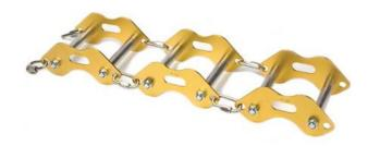
Three linked units with hard anodized aluminum side plates and two roller bars each. This lightweight and compact roller can be used linked together with the furnished screw links at sharp edges, or separated for long gradual breakovers.
