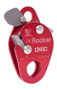
The ISC Rocker, can be fitted to the rope at any point and can be used hands-free as a self-tailing device when travelling up or down the rope. The ISC Rocker, Ropegrab for Rope Access back up is designed for use without a shock-absorber and can be used as a Rope Adjuster or on a work positioning lanyard/Flipline, (In accordance with EN358). Use 10.5 mm to 11.5 mm rope with the ISC Rocker, DECLARATION OF CONFORMITY All items in the Outlet are considered final sale.
