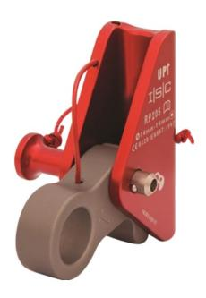
The ISC Large Ropegrab is fitted with a pip-pin axle, making it quick and easy to attach/detach mid-line. A thumb operated push-button is used to disengage the Pip-pin mechanism and the axle has a chamfered end, to allow for easy location of the pin. The ISC Large Ropegrab has a textile Pip-pin retention cord, (rather than a wire cord). The textile cord allows for easy maneuvering of the pin and does not snag, or wear with sharp edges.
