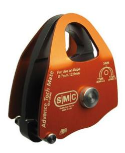
The new SMC Advance Tech Mate is a double pulley specifically designed to work with the new Advance Tech HX Pulley in a mini haul system. This new pulley frame design is ideal for using in a compact haul kit. Integrated stainless steel pins help retain the rope when a rigged system is pre-packed in order that the system can be pulled out and used immediately.
