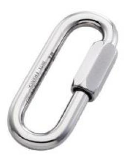
Screw links stand up to multi-directional forces better than carabiners and allow ample room for multiple pieces of gear to be attached. Ideal harness attachment in ascending systems or for joining anchor straps. The original oval shape was developed on the principle of a chain link fitted with manual nut opening. Made in France by Maillon Rapide.
