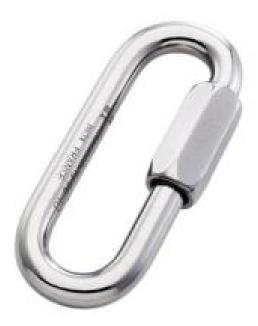
Screw links stand up to multi-directional forces better than carabiners and allow ample room for multiple pieces of gear to be attached. Ideal harness attachment in ascending systems or for joining anchor straps. *Note: Links are stamped with a Working Load Limit (WLL) that is about 1/5 of its rated breaking strength.*
