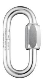
Screw links stand up to multi-directional forces better than carabiners and allow ample room for multiple pieces of gear to be attached. Ideal harness attachment in ascending systems or for joining anchor straps. *Note: Links are stamped with a Working Load Limit (WLL) that is about 1/5 of its rated breaking strength.*
