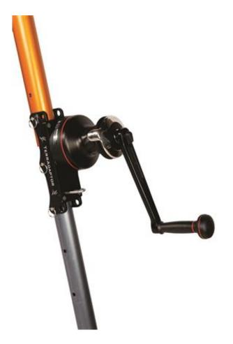
The new SMC TerrAdaptor<sup>™</sup> Capstan Winch System mounts on any grey leg tube section in any position on the TerrAdaptor<sup>™</sup> multi pod. A stainless steel rope guide ensures that the rope enters the capstan at the correct angle for the greatest grip. Clip points on the front and rear of the bracket can be used for progress capture devices such as a rope grab or a prusik.
