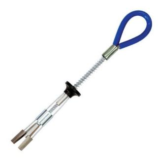
This anchor can be removed and reused at any desired location. It features unmatched safety, ease of use, and speed. The RB Anchor works in horizontal, vertical, and overhead/ceiling surfaces. Costly engineering inserts are not required. This anchor can be used for fall protection, restraint, work positioning, and more. This product is designed for use in concrete or rock only.
