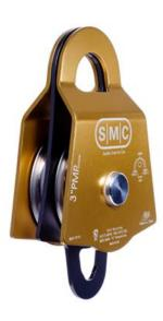
The unique shape of SMC's aluminum side plates allow the efficient use of Prusik hitches as a belay or progress capture device. Constructed with a 3" diameter sheave running on a high efficiency ball bearing. Low profile fasteners help eliminate the possibility of the pulley snagging. Pulley will accommodate up to 13 mm rope.
