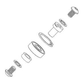
To maintain peak performance the bearing assemblies on the Shuttle Xtreme can be replaced by the user in just 4 steps with the new Cable Xtreme Service Kit or Rebuild Pack. The Xtreme Service Kit (SKU SM156309) comes with all the necessary parts and tools needed to rebuild a single unit. The Xtreme Rebuild Pack (SKU SM156308) comes with all the parts needed to rebuild up to 10 pulleys (tools not included).
