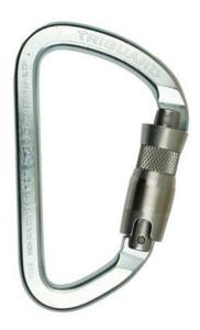
A Lite Alloy steel carabiner featuring double or triple action gates. Easily opened with one hand, but once released, the gate closes to a fully locked position. The carabiner gate and sleeve are stainless steel for problem-free operation. An offset "D" shape provides a smooth transfer of the Munter hitch when used as a belay and has ample volume to clip in large diameter ropes and over the rails of most litters.
