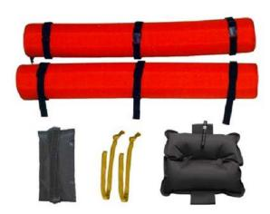
This self-righting flotation system maintains the Sked® in a nearly vertical position even in rough water. Two rigid foam side floats and an inflatable chest bladder provide buoyancy sufficient to support two rescuers in addition to the patient.
