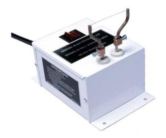
Fusing rope ends helps protect your rope and prevent unraveling after cutting the rope.
