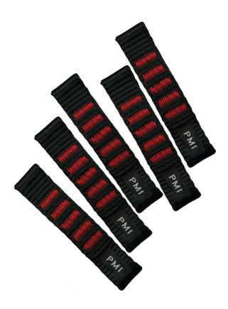
These sewn polyester Short Links are built with super 18 mm webbing for optimum carabiner loading while maintaining a high 22kN breaking strength.
