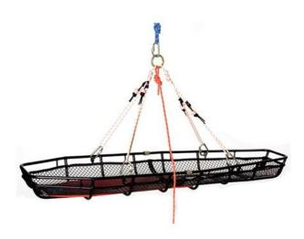
Adjustable 4 leg litter spider made from 10 mm PMI® Classic static rope and 6 mm prusik cord tied on a forged O-ring. Litter and carabiners in photo not included.
