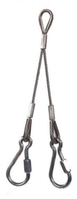
Used when you need to attach a flexible ladder to a single attachment point. A LADDER SPREADER is used to link the ends of a COMPACT flexible sided ladder to a suitable anchorage. Its Y shaped construction achieves the correct loading angle on the COMPACT ladder ends where the ladder is rigged from a single anchor point. *Note: LADDER SPREADERS are not PPE. They must not be used as an alternative to an EN795 wire anchor strop.*
