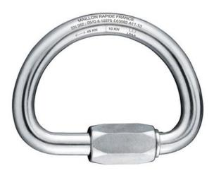
Screw links stand up to multi-directional forces better than carabiners and allow ample room for multiple pieces of gear to be attached. Ideal harness attachment in ascending systems or for joining anchor straps. The Half moon (semi-circular) shape is suitable for the junction of 2 connecting points on a harness. Made in France by Maillon Rapide.
