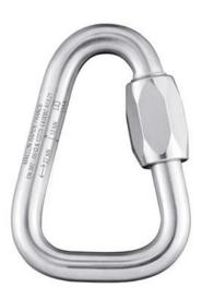
Screw links stand up to multi-directional forces better than carabiners and allow ample room for multiple pieces of gear to be attached. Ideal harness attachment in ascending systems or for joining anchor straps. *Note: Links are stamped with a Working Load Limit (WLL) that is about 1/5 of its rated breaking strength.*
