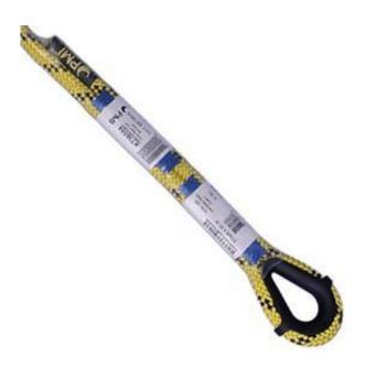
PMI uses precision stitching to create a permanent, sewn termination that is stronger than any knotted termination and nearly as strong as the rope itself. Heat shrink tubing protects the stitching and the label from abrasion. PMI can sew either one or two end terminations on the following ropes and these are certified as Manufacturer Supplied Eye Terminations per NFPA 1983:2012:
