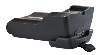
Powerful battery to extend the <u>ACX POWER ASCENDER kit</u> (SYPOA-001) when more than two batteries are required for one device. The quick-charging battery has an electronic management system with LED display that provides information on its charge status at all times. With a user load of 100 kilogrammes, one battery charge is sufficient for up to 200 metres of rope. At higher weights, the battery performance is correspondingly somewhat lower.
