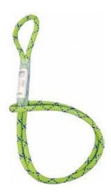
PMI® is proud to offer the latest innovation in accessory cords. Precision sewn loops form a sleek, low profile connection that is stronger than a knot. Clear tubing protects the stitches yet allows for easy inspection. Built for those looking for a no-Knot solution for prusik minding pulleys. These Pre-Sewn prusiks work great in hauling systems that require a prusik load capture, the sewn prusik is always stronger and more reliable than a tied knot prusik. Also available in 6 mm and 7 mm.
