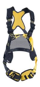
A very light and compact fall arrest harness with 2 connection points: 1 sternal and 1 dorsal. Quick release buckles to the thighs and a foamed back allow a quick sitting. Versatile because it can be combined with a work position belt.
