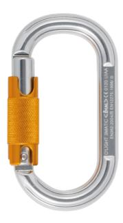
O'LIGHT is a symmetrical aluminum triple locking screwgate carabiner. Its oval shape has been designed to easily connect double flange equipment such as pulleys, blockers, mobile fall arresters for example. It also has a keylock system and each carabiner has an individual number that guarantees its traceability.
