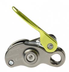
The BIRDIE is a brake-assisted belay device. Compact, it is also ergonomic for a better grip. It can be used with all dynamic single ropes, with a diameter of 8.5 to 10.5mm. Each of Beal's belayers has an individual number that guarantees its traceability. Entirely made of metal, with cam and friction components in stainless steel for great durability. The rope exits following the device's axis, to avoid twisting.
