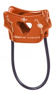
The AIR FORCE 1 belay device can be used with single ropes of a diameter between 8.5 and 10.5 mm. The V-groove runs smoothly enough to pay our slack easily, but also offers extra friction to improve rope braking while belaying and optimum energy absorption should the climber fall. The wide, smooth groove also avoids parasitic friction on edges and keeps rope wear to a minimum. For added security, each belay device has an individual number that guarantees its traceability.
