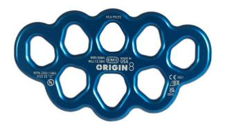
Origin 8 large rigging plate, boasts the perfect quantity of connection points to ensure orderly rigging and serves as an excellent choice as a master point for litter bridles. Its generous connection apertures enable seamless rotation of most locking carabiners. This robust plate exhibits an impressive Minimum Breaking Strength (MBS) of 50kN in all directions and is meticulously crafted with specialized tooling to provide rounded edges that are gentle on textiles.
