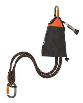
A self-locking hauling system featuring a 4:1 mechanical advantage, or 5:1 when inverted, designed for optimal performance in rescue scenarios. Specifically crafted for the lifting and release of injured operators or effective tensioning of a rope system.
