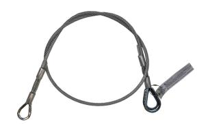
The slings are excellent temporary and semi-permanent ANSI-certified anchors. The breaking strength of 5000 pounds allows for versatility on the job or in a rescue kit. Clear tubing makes for easier cable inspections.
