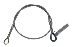
The slings are excellent temporary and semi-permanent ANSI-certified anchors. The breaking strength of 5000 pounds allows for versatility on the job or in a rescue kit. Clear tubing makes for easier cable inspections.
