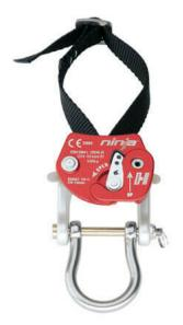
The Ninja MultiAscend is engineered to provide increased efficiency in a range of applications. The dual cam design enables the MultiAscend to act as both a chest ascender as well as a full point of attachment. The innovative dual-stage locking swingplate ensures consistent engagement with the rope, preventing unwanted detachments. In addition, the external release triggers make adjusting the Ninja MultiAscend safe and easy when used as an ascender or a progress capture device on a safety line.
