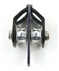
The Micro Hauler Double Pulley with becket is a tiny but extremely strong and efficient version of the Rescue Black andoized alumimum sideplates, two 1 1/4" aluminum sheaves, bushing and aluminum axle. Hauler. 7,000 Ibs MBS, 1/2" Rope Capacity, 3.5 x 1.75 inch, 133.6% Efficiency, 6" Length, 1" Sheave Diameter. When the Micro Hauler (SK-710-M) is used with the matching double pulley SK-712-M, it gives you a 4:1 mechanical advantage.
