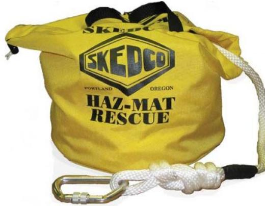
HMH Shuttle Sked rope is constructed of 1/2 inch solid braid polypropylene. It is 200ft. long with a figure 8 knot saftied with a barrel knot and taped to prevent unraveling while in use. A Large aluminum D carabiner is attached. The rope kit includes a Haz-Mat rope bag for quick tangle free deployment. This rope is attached to both ends of a HMH Sked for dragging into and out of the Hot-zone. We suggest two rope kits for each HMH Sked to operate efficiently in the hot-zone.
