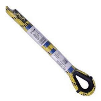
PMI uses precision stitching to create a permanent, sewn termination that is stronger than any knotted termination and nearly as strong as the rope itself. Heat shrink tubing protects the stitching and the label from abrasion. PMI can sew either one or two end terminations on the following ropes and these are certified as Manufacturer Supplied Eye Terminations per NFPA 2500 (2022).
