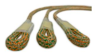
These prusiks feature eye-to-eye construction with a durable 8mm Technora sheath over a light-weight high strength Dyneema-based core. This light weight, abrasion resistant static cord repels water and handles great under the most challenging conditions.
