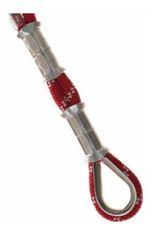
High strength, no-knot terminations for PMI® Hudson Classic ropes. PMI swaged rope terminations are always stronger than any knotted termination. Swaged terminations are formed using aluminum sleeves and a stainless steel thimble. Swages are applied to the rope using a precision steel die and the resulting termination is nearly as strong as the rope itself. (Ropes may not be swaged after leaving the factory.)
