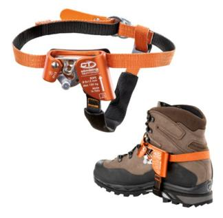
The Climbing Technology QUICK STEP-A Ascender for the right or left foot which, used in conjunction with an ascender handle (e.g. <u>QUICK'UP</u>) or a chest ascender (e.g. <u>CHEST ASCENDER EVO</u>), makes it easier and speeds up the ascent a rope. Ideal for working at height and tree climbing, it is equipped with an opening lever which allows you to keep the device open to facilitate insertion of the rope and prevent it from accidental slipping out.
