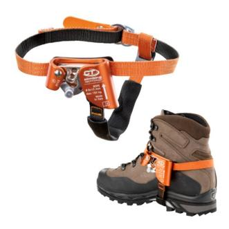
The Climbing Technology QUICK STEP-A Ascender for the right or left foot which, used in conjunction with an ascender handle (e.g. QUICK'UP) or a chest ascender (e.g. CHEST ASCENDER EVO), makes it easier and speeds up the ascent a rope. Ideal for working at height and tree climbing, it is equipped with an opening lever which allows you to keep the device open to facilitate insertion of the rope and prevent it from accidental slipping out.
