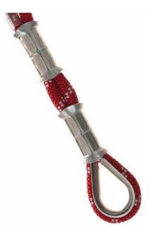
High strength, no-knot terminations for PMI® Classic and Patriot ropes. PMI swaged rope terminations are always stronger than any knotted termination. Swaged terminations are formed using aluminum sleeves and a stainless steel thimble. Swages are applied to the rope using a precision steel die and the resulting termination is nearly as strong as the rope itself. (Ropes may not be swaged after leaving the factory.)
