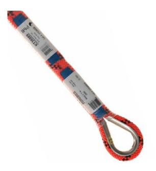
PMI uses precision stitching to create a permanent, sewn termination that is stronger than any knotted termination and nearly as strong as the rope itself. Heat shrink tubing protects the stitching and the label from abrasion. PMI can sew either one or two end terminations on the following ropes and these are certified as Manufacturer Supplied Eye Terminations per NFPA 2500 (2022).
