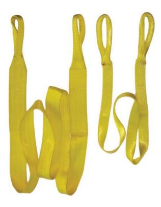
The Skedco Soft Anchor Sling is a perfect utility strap suitable for many purposes. With loops sewn on each end, this strap is lightweight and easy to use. The 6 ft model is constructed of 16,000 lbf tensile strength webbing and the 8, 12, and 20 ft long models are of 20,000 lbf webbing.
