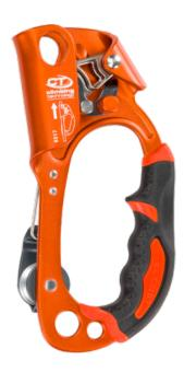
The Climbing Technology QUICK ROLL is designed with a new ergonomic handle ascender for greater efficiency when pulling. Cam opening lever usable with one hand Steel cam, resists wear and tear. The QUICK ROLL is available for left-hand or right-hand. Innovative handle ascender with integrated pulley. Used in conjunction with a self-braking descender (Climbing Technology SPARROW) it allows for ascending the work rope. Ideal for placing protection and for rock scaling on crags.
