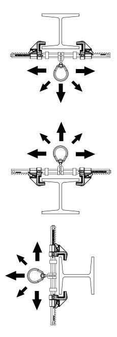
Placement at or below a user's working height requires integration of a compatible ANSI Z359.1 shock-absorbing lanyard that does not allow the user to extend more than 6 feet (in any direction) from the anchorage connector before the shock absorber is activated. The beam anchor must be attached to the l-beam flange facing the user (top flange if above, bottom flange if below, etc.).
