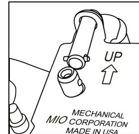
5. Make sure that locking pin balls appear on outside of main assembly and the direction arrow on the housing is pointing up.
