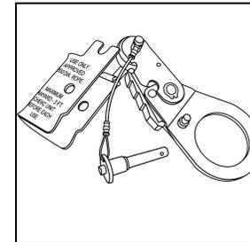
2. Swing cam and lever assembly up and open.
