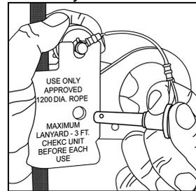
4. Close assembly, align holes and reinsert safety locking pin.
