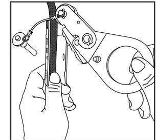
3. Place rope grab on rope with plastic roller pointing up.
